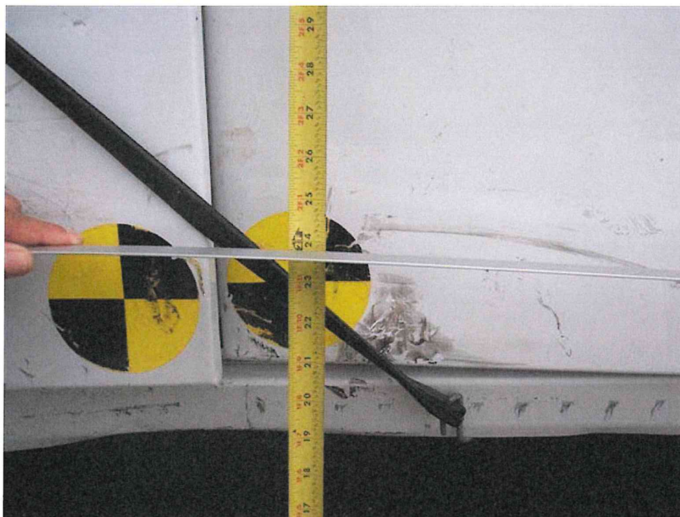
LEFT SIDE IMPACT SHOWING MEASUREMENT OF MAXIMUM CRUSH (TEST #055)
