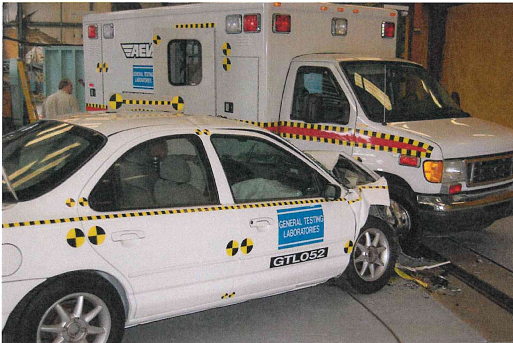
GTL TEST #052 – POST TEST
