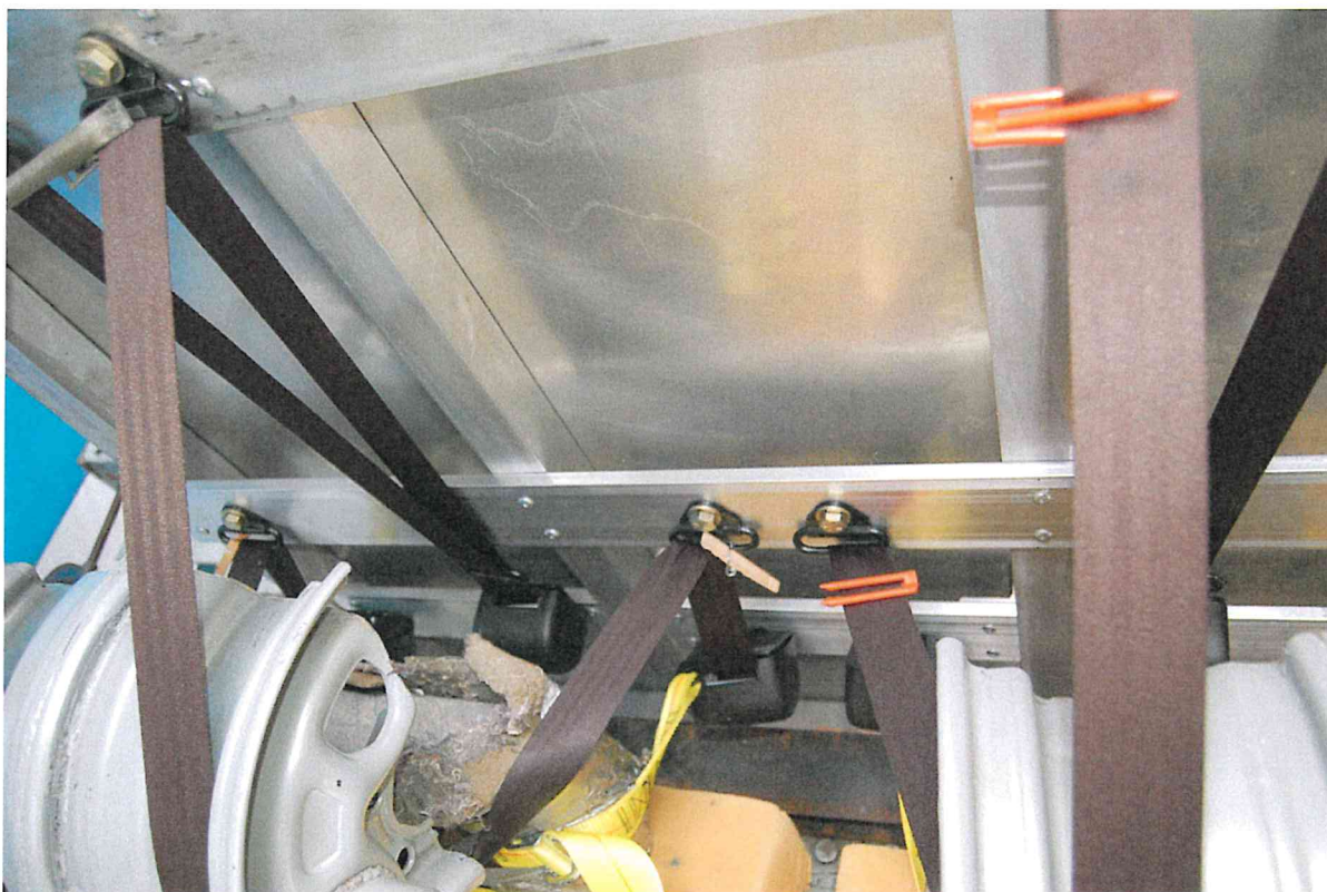
TEST #6627 - 210 POST TEST BELT MOUNTING
