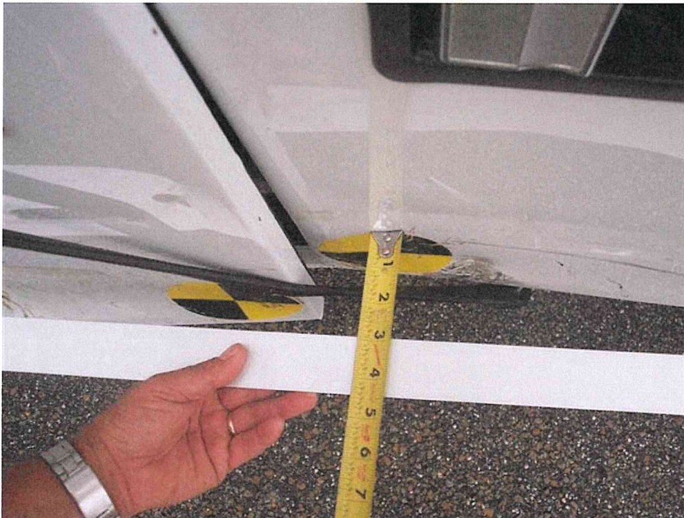
LEFT SIDE IMPACT SHOWING MEASUREMENT OF MAXIMUM CRUSH (TEST #055)
