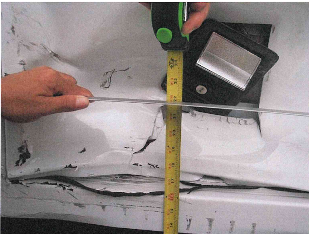
RIGHT SIDE IMPACT SHOWING MEASUREMENT OF MAXIMUM CRUSH (TEST #052)
