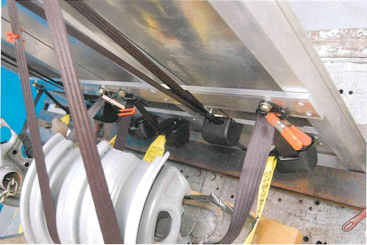
TEST #6627- 210 POST TEST BELT MOUNTING
